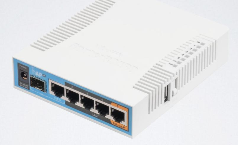
Dual band 2.4/5GHz AP, 802.11ac/a/b/g/n, 5x1Gbps Ethernet, PoE-out on port 5, SFP and USB
