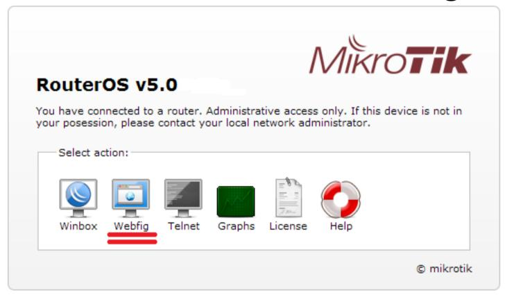
WebFig is a web based RouterOS configuration utility. It is accessible directly from the router
